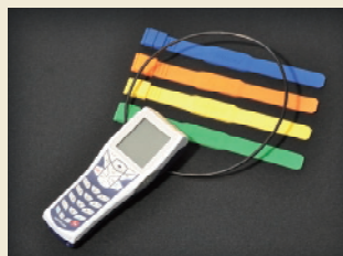
A wristband for entrance/exit management using RFID
