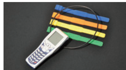
A wristband for entrance/exit management using RFID
